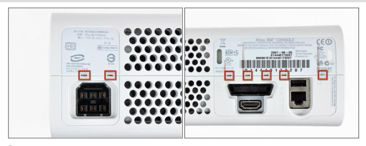
The upper and lower cases are held together by seven release latches located on the back of the console. Their locations are highlighted in red.
