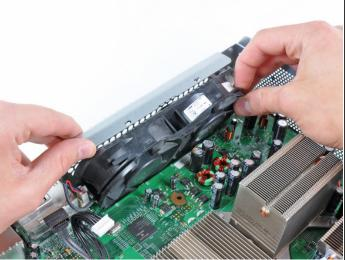
While lifting the metal chassis strip above the dual fans, pull the fans toward the center of the motherboard.
