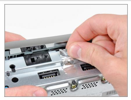
Peel the silver tape securing the optical drive to the metal casing.
