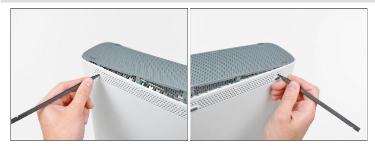
• Use the tip of your spudger to release the clips on the bottom vent nearest the back of the Xbox.
