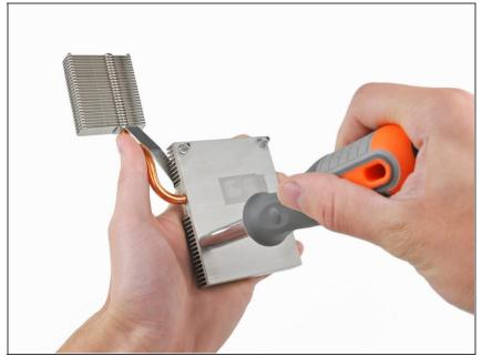
Use the 1/4" drive end of the included 6-in-1 screwdriver with no bit inserted to remove the four Xclamp posts from both the CPU and GPU heat sinks.
