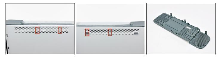
in the next few steps, you will use the tip of a spudger or the finger of an Xbox 360 opening tool to release the clips along the left and right sides of the top vent. Their locations are highlighted in red.
