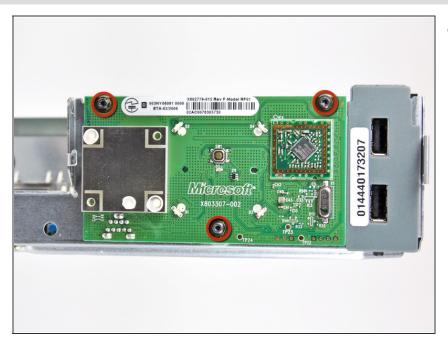
Remove three 5.6 mm T8 Torx screws securing the RF module to the metal chassis.
