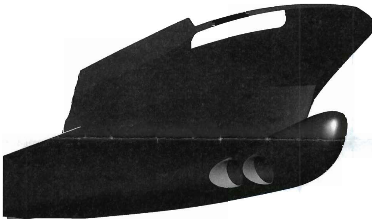
Figure 2: Bulbous Bow 3D Model
